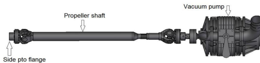
FIGURE 64: SCHEMATIC REPRESENTATION OF VACUUM TRUCK WITH 4 CUM CAPACITY AND ITS VACUUM SYSTEM AND DRIVE SYSTEM
