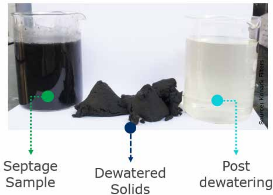
FIGURE 68: PICTURE DEPICTING THE INFLUENT AND EFFLUENT OF A DEWATERING TRUCK
