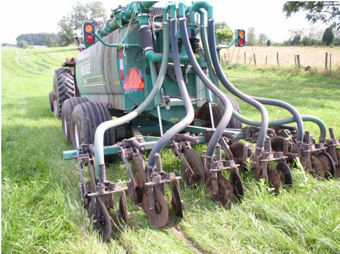
FIGURE 74: EQUIPMENT REQUIRED FOR SUB SURFACE INCORPORATION (SOURCE: SOURCE: R. MAGUIRE, VIRGINIA TECH)
