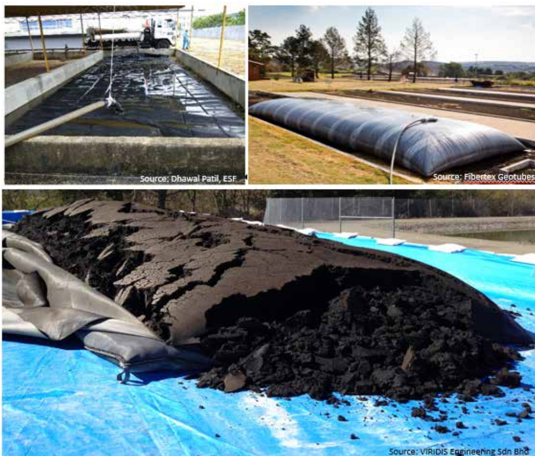
FIGURE 77: PICTURES OF GEO TUBES AT VARIOUS STAGES
