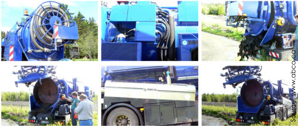
FIGURE 69: PICTURE OF A DEWATERING TRUCK FITTED WITH MECHANISED DEWATERING EQUIPMENT
