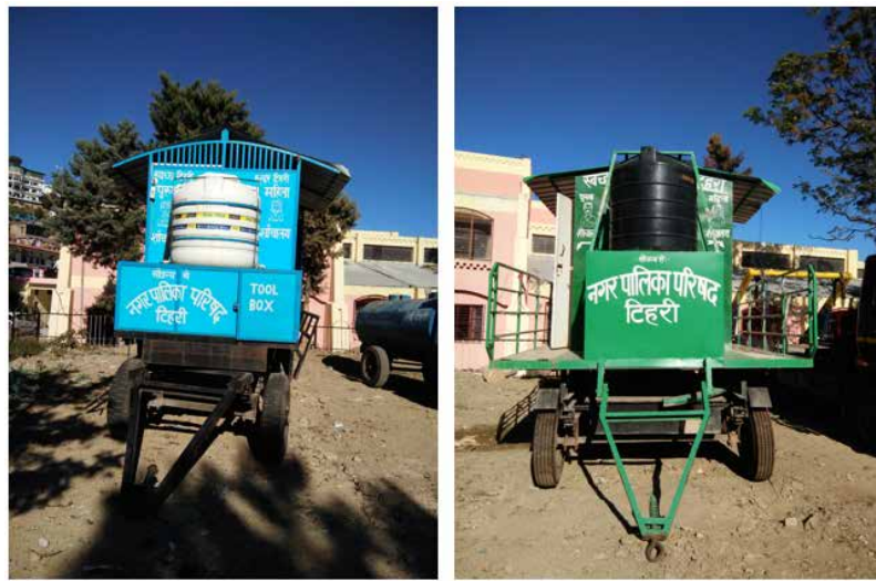
FIGURE 24: MOBILE TOILETS EQUIPPED WITH WATER STORAGE AND LIQUID WASTE STORAGE TANKS, TEHRI NPP
